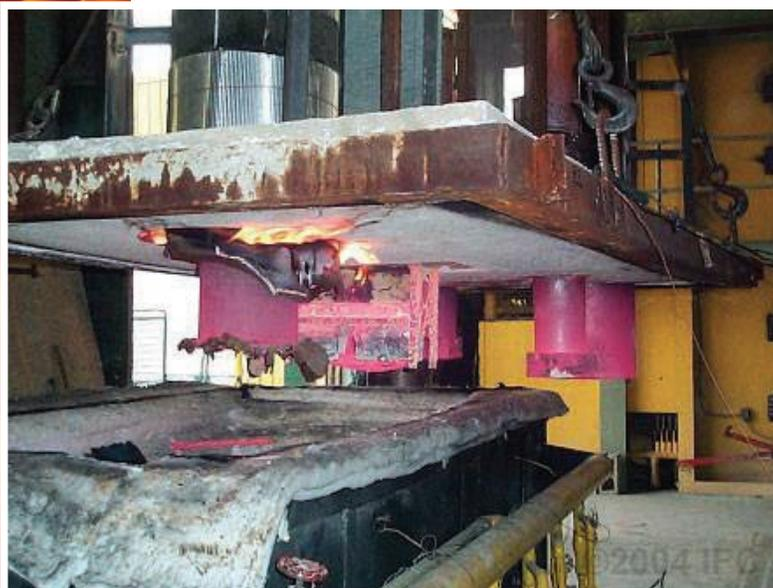
Figure 1 Assemblies are tested in a furnace to determine their fire rating.
