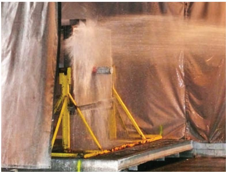
Figure 2 Assemblies are subject to a hose stream test to determine overall integrity.
