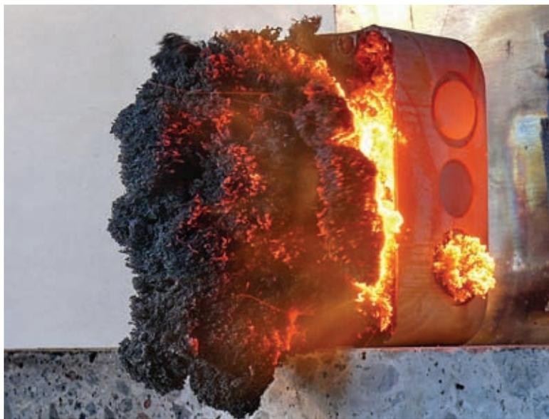
Figure 3 An intumescent electrical box insert
