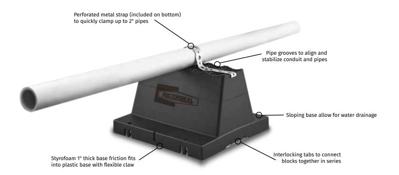
Dimensions: 8" x 7.5" x 5" Load Rating: 200 lbs. 250 lbs. with strut
